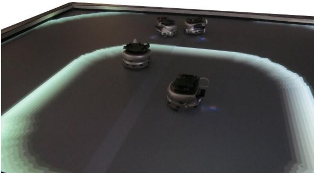
Figure 7: Snapshot of an experiment using the Khepera robots on the interactive ROMEA table. The experiment uses a circular neighborhood with radius 2.5 and  $M=6$
